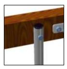
10 With the gearbox handle, wind the curtain up to the side rail. Fix the top end of the guide tube to the side rail with an M8 x 50 coach screw. Fit a PVC plug into the top end of the guide tube.
