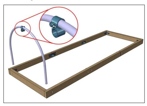
6 Slide the ridge tube(s) into the E25 fittings. Gently tighten the M8 bolt in each fitting. Your framework is now complete.
