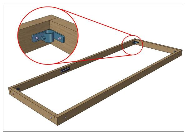
4 For mini polytunnels 8ft long, 10ft long and 12ft long, drill and bolt the H25 fittings to the length timbers. For the 8ft long and 10ft long mini polytunnels, these are at mid-length. For the 12ft long mini polytunnels, these should go over the timber joint plate where the two timbers join (at approximately 114cm from each end).
