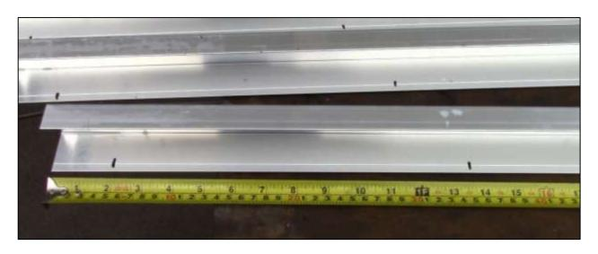
Tip! Rest the Aluminium Gutter on a piece of wood while drilling the holes to minimise the burr.
